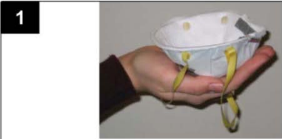
Cup the respirator in your hand with the nosepiece facing your fingertips and the straps hanging below the hand.
