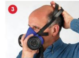
3 With your other hand, position the plastic straps so they are centered on your head. Remove any slack in the upper straps by pulling the two end tabs back and toward your ears. DO NOT TIGHTEN AT THIS TIME.
