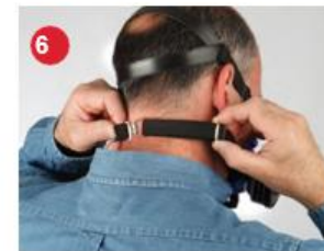
6 Tighten the lower head straps by pulling evenly on the end straps in the back of the respirator until the entire respirator is snug, comfortable and centered on your face.
