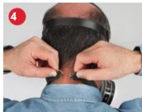
4 Fasten the bottom elastic straps behind your neck and under your hair. Remove any slack in the bottom straps by pulling the end tabs in the back towards the front. DO NOT TIGHTEN AT THIS TIME.
