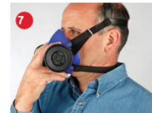
7 Gently pull the respirator away from your face and maneuver it to assure it is centered, comfortable and snug. Plastic loops on the top straps slide back to hold down any loose strap material.
